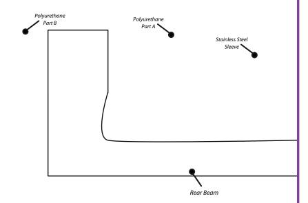
Figure 1 - line drawing of how the polyurethane parts fit together
