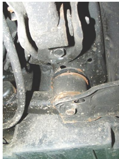
Figure 1. Original Rear Subframe Mount
