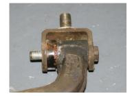
PFR17-207W fitted in the same way as PFF17-201 with top-hat section installed towards centre of wishbone. Note washer locations.
