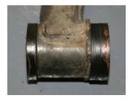
PFR17-209 fitted similar to PFF17-201. It is important to retain the original heatshield and re-apply it after fitting the POWERFLEX bush. If the original heatshield is no longer present, ensure a replacement heatshield is fitted. Note washer locations.
