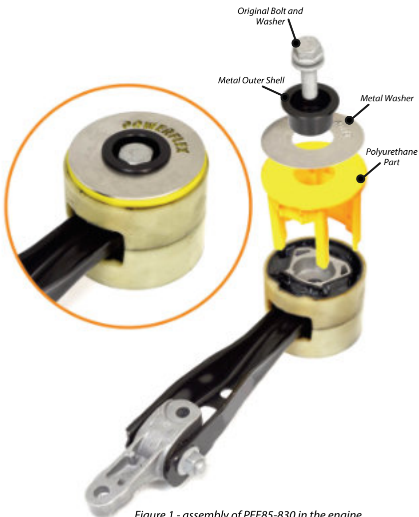
Figure 1 - assembly of PFF85-830 in the engine mount
