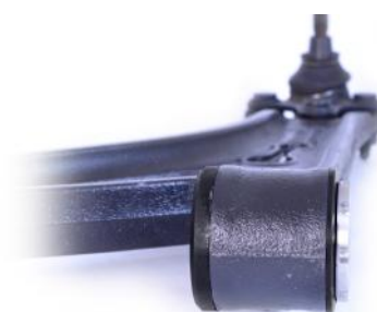
Figure 1: B Bush shown Inserted from the front of the wishbone
