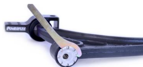
Figure 2: Sleeve positioned towards the middle of the car for maximum camber
