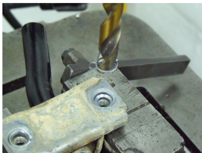
Figure 2 - Removal of the swaged section of the bracket.
