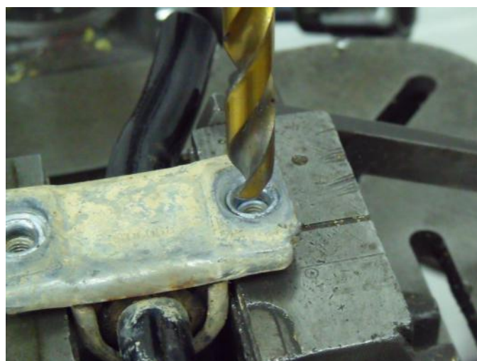
Figure 1 - how to remove the swaged section from the bracket
