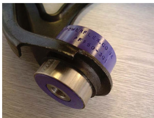
Figure 1- Bush fitted in wishbone
