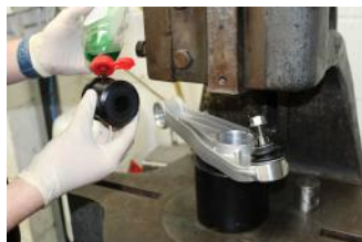
1. Applying Washing Up Liquid
