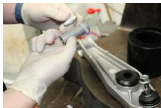
4. Applying the PTFE Grease
