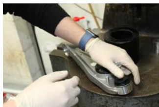
5. Pressing the Stainless Steel Sleeve
