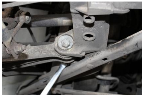
Figure 2 - Remove the inner bush bolt
