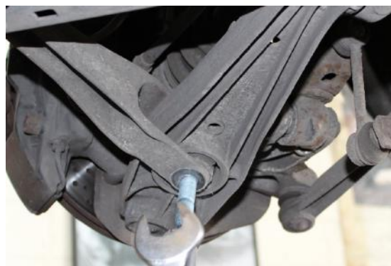
Figure 1 - Remove the outer bush bolt securing control arm link to arm
