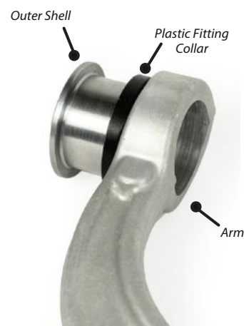
Figure 1 - Orientation of Fitting Collar, for pressing the Rear Bush
