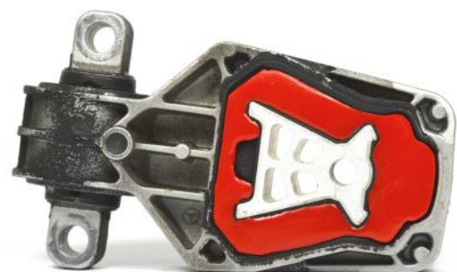
Figure 1 - showing polyurethane insert fitted inside the lower engine mount
