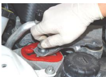
Figure 4 - showing polyurethane insert fitted inside the top engine mount
