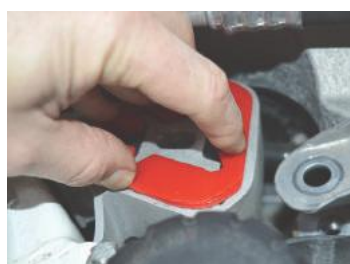
Figure 3 - exploded view showing how the insert fits inside the top engine mount
