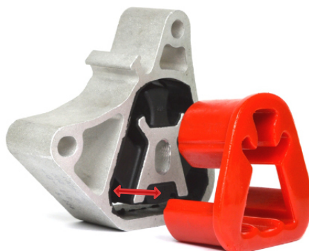
Figure 3 - exploded view showing how the insert fits inside the top engine mount
