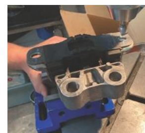
Figure 2: Drill swaged holes
