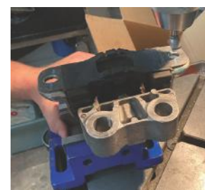
Figure 2: Drill swaged holes
