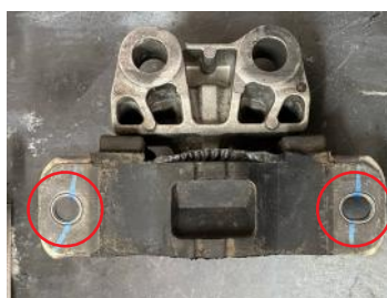
Figure 1: Swaged bolt holes to be drilled
