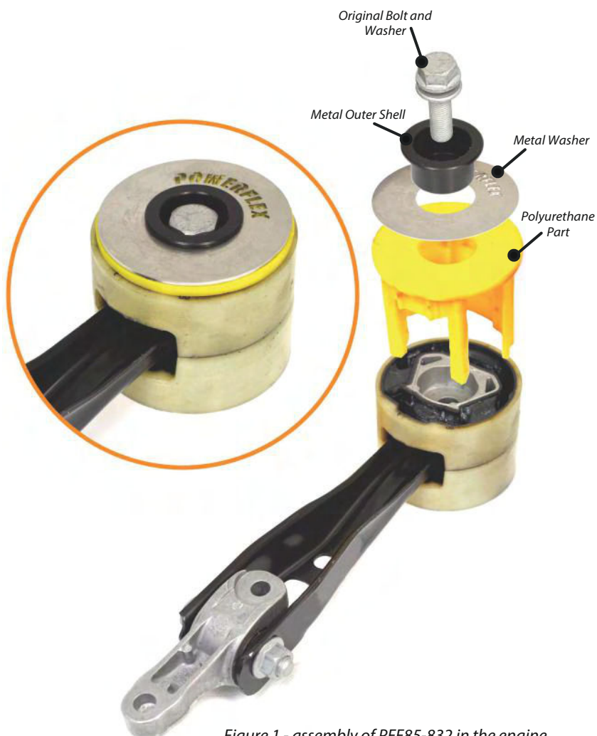
Figure 1 - assembly of PFF85-832 in the engine mount
