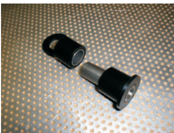
79-102H Single part showing glacier bearing
