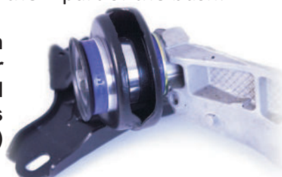
B Bush Outside of car (Original domed washer goes here)
