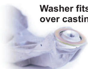
B Bush Outside of car (Original domed washer goes here)
