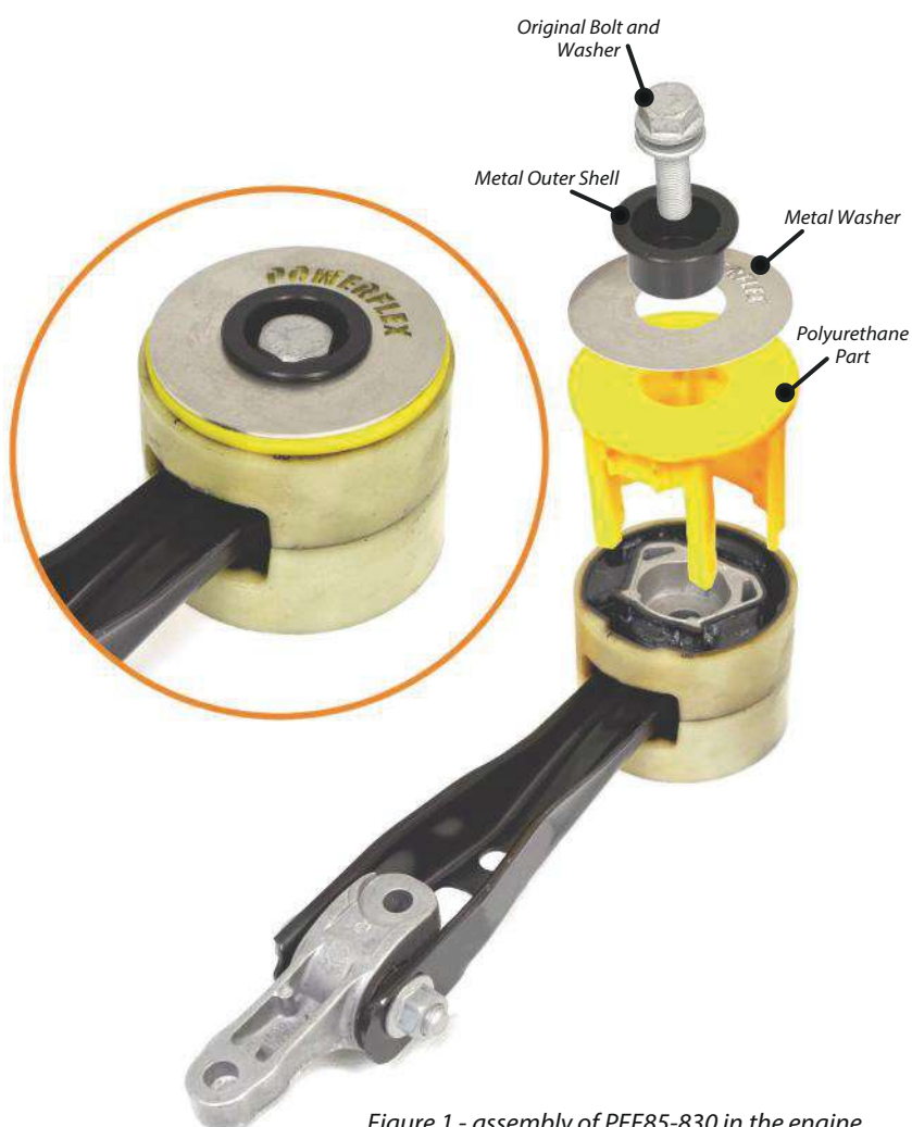
Figure 1 - assembly of PFF85-830 in the engine mount
